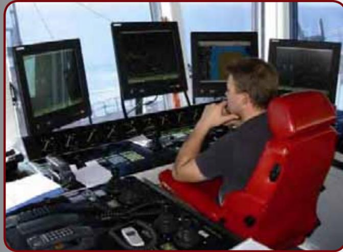
Dredge display with underwater bathymetry; the dredger has one suction pipe on the seabed. The position of the draghead is perfectly known in three dimensions. Accuracy of the work is often one or two metres, horizontally.
